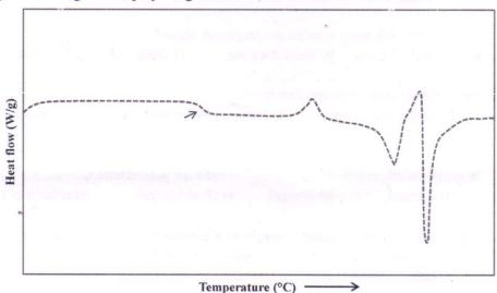
a) Glass transition temperature,d) decomposition temperature
